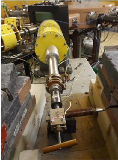
The view of our portable high-pressure apparatus located in the Mikrotron MT25 electron accelerator system in the Dubna Nuclear Reactions Laboratory JINR. A fragment of the accelerator installation is visible. Completely working equipment of accelerator was in perfect state during our, long-term, cooperation.
