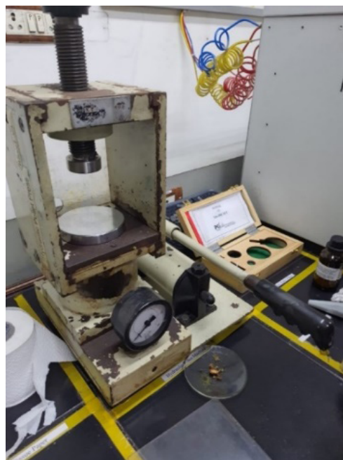
Figure 1: Hydraulic Press machine to prepare KBr Pellet.
