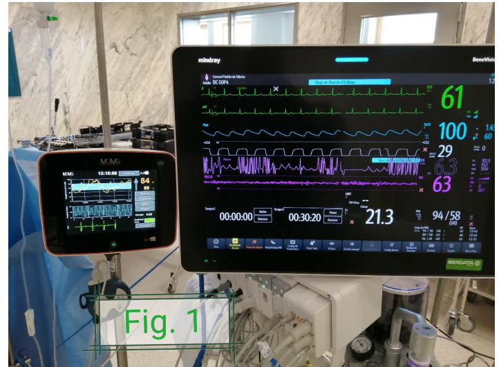
Figure 1: The Opioid Free Anesthesia goal-directed strategies are based on monitoring: ECG; ANI; ICG; TOF; BIS.
