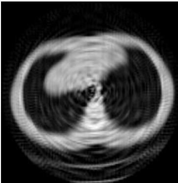
Figure 18: Reconstruction from linear-interpolated sinogram.
