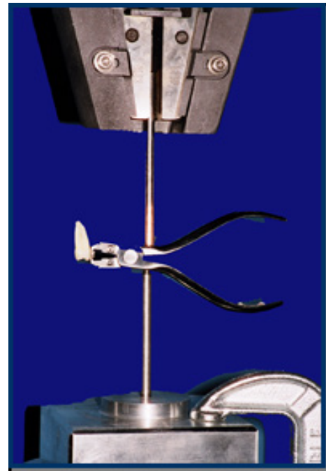
Figure 4: Compressive load applied by the Instron machine on the pliers arms.
