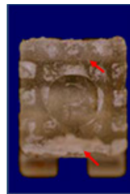
Figure 9: Un-fractured bracket base after debonding. Red arrows represent fractured tiny mechanical projections.
