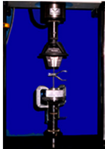
Figure 2: Debonding plier mounted on the Instron machine.
