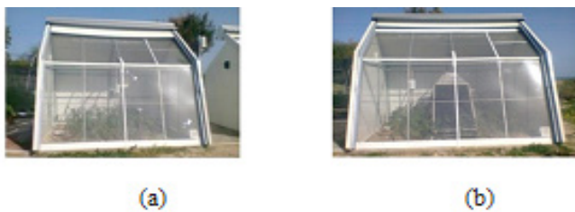
Figure 1: Photo of the experimental greenhouses: (a): Insulated greenhouse (IG), (b): Insulated greenhouse with latent heat system (IGHLS).
